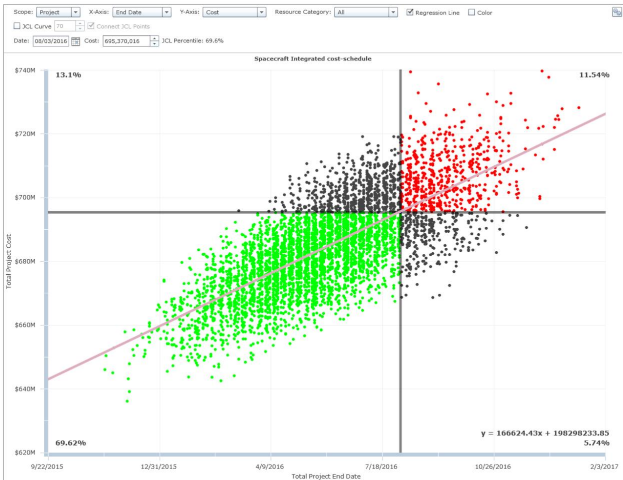
Figure 2 Scatter Diagram Illustrating Finish Date and Cost Results
